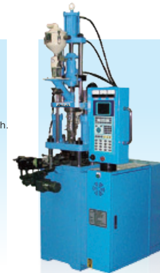
■ 拉鏈機 Zipper machine 自動送帶、收帶上下一次為一次成型。 Automatic strap feeding and take-up for one-time injection.
