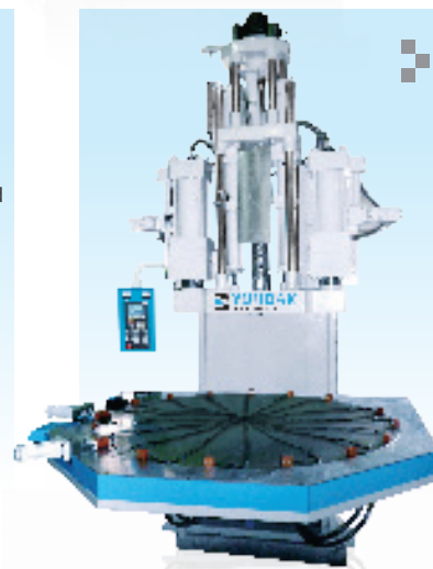
■ 插頭專用機 Plug making machine 適用一般電器插頭，電子零件等小型嵌件成型。 Suitable for general electrical plugs, electronic components, and other small embedded pieces of molding.
